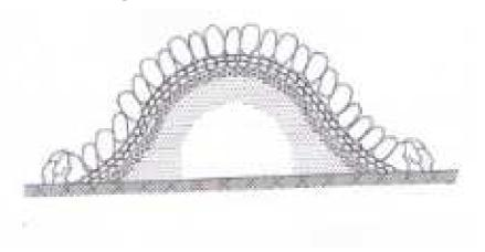
Fig. 14.2. A Rubble mound breakwater
